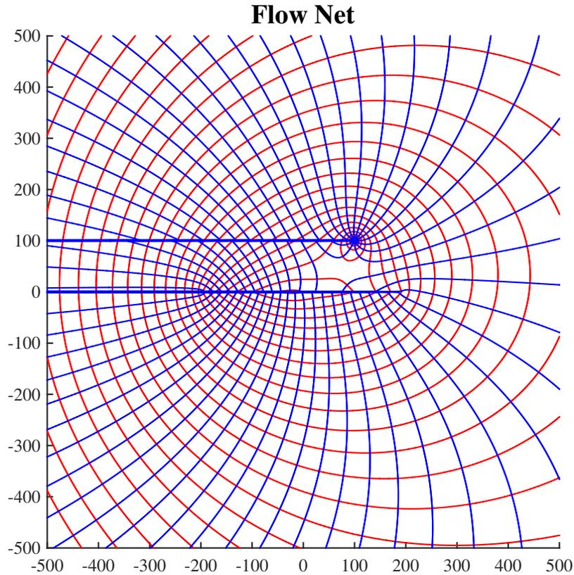
Figure 1: Discharge Potential and Streamline Contours
