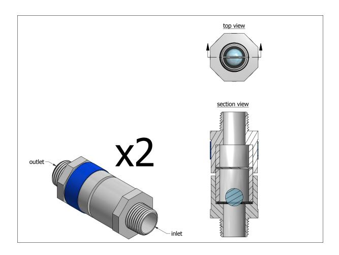
**Total Parts Needed for Assembly of 2 Check Valves**
