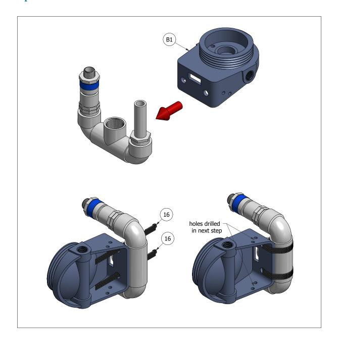
Using hose clamps, attach filter bowl head to assembly. Use whatever mounting holes are already present on head.
