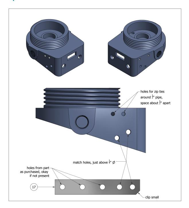
Drill holes in head and any rigid metal strip such that when attached, the assembly rests upright. If needed, clip strip corners to avoid interference.
