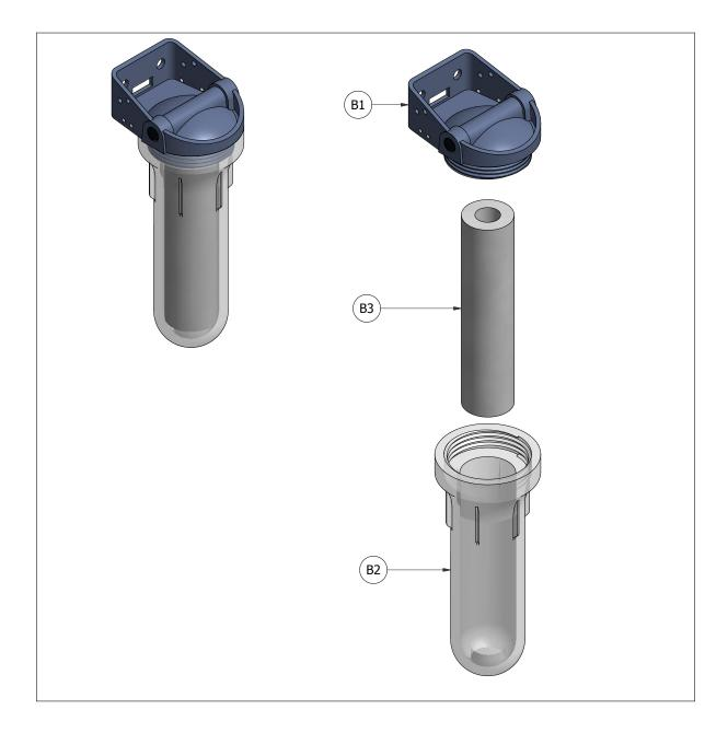
Separate parts of filter bowl. Head will be used first, with cartridge and bowl added later.
