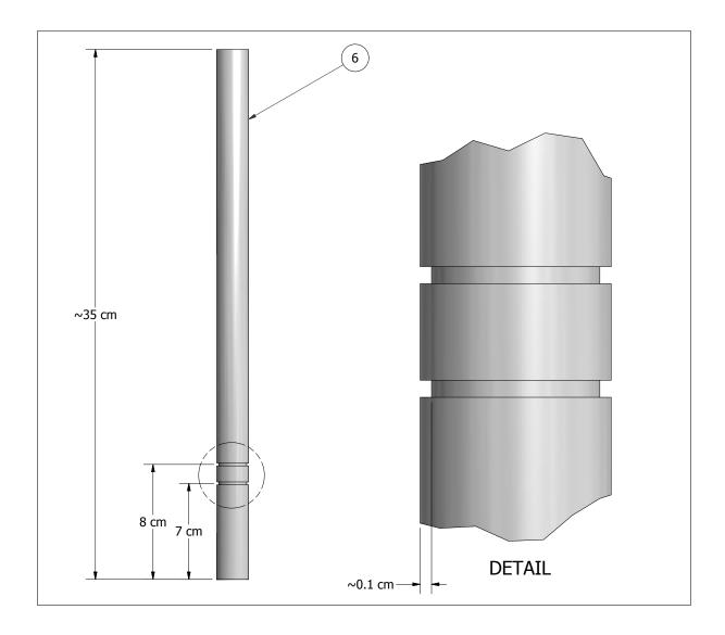
Using a table saw, lower blade such that very little of the wheel's teeth protrude above the work surface. By shifting pipe over these teeth and rotating, create very minor recess along exterior surface, as shown.
