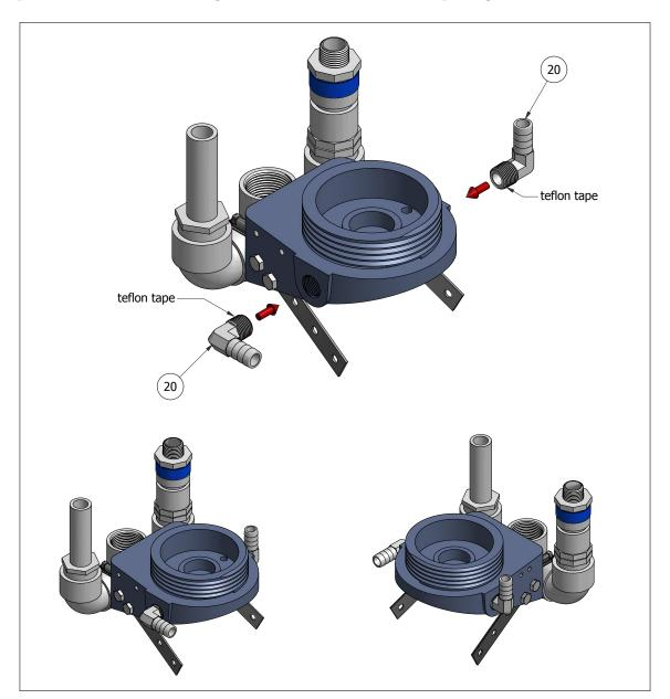
Step 15: Insert barbed fittings into both filter bowl head openings.
